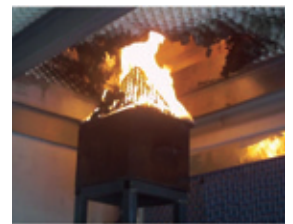
Heptane ignition source for full-scale fire testing
