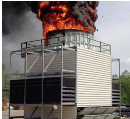
Minimal damage from successful ESP full-scale fire test. Franklin Fill™ material chars inhibiting the spread of fire
