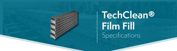
**TechClean®** is a low fouling film fill with vertical offset flutes, to reduce fouling but with a high wetted surface area for maximum heat transfer. The sheets are manufactured from rigid PVC and meet CTI Standard 136. Solvent bonding produces modules that can withstand severe installation handling as well as operational and maintenance situations. TechClean is resistant to UV.
