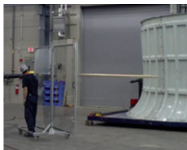
Airborne debris (missile) testing
