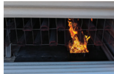
Heptane ignition source for full-scale fire testing
