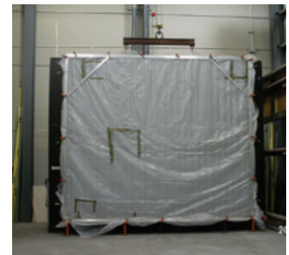
SafeWall™ cyclic wind pressure testing
